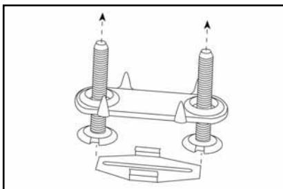
**4.** For 2-1/2, 3, 1-1/2FP, 2FP, RP1, and RP2, assemble bottom plate. Insert 2 bolts and attach clip.
