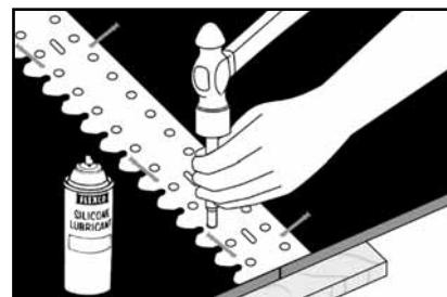
**3.** Spray templet holes with Flexco Silicone Lubricant. Punch or bore bolt holes. Remove templet.
