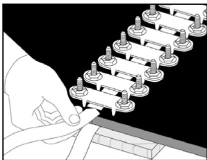
**9. Cut Flexco-Lok® Tape 3-1/2 times the belt width and feed tape under top plates, under the bottom plates, then back under top plates.**
