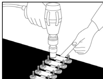
**10. Pull tape tight and hold in position by tightening a fastener at each end. Then tighten all other plates.**
