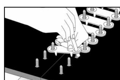
**7.** Place top plates over bolts using bolt horn.
