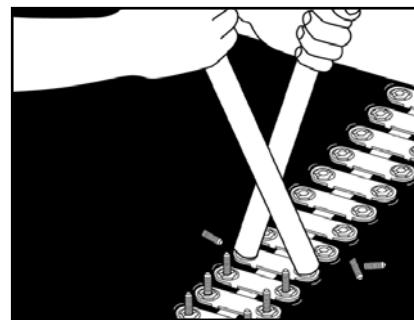
**11. Tighten all fasteners from edges to center. Tighten all nuts uniformly. **NOTE:** A Flexco Power Wrench used with an impact tool will speed this step considerably.**
