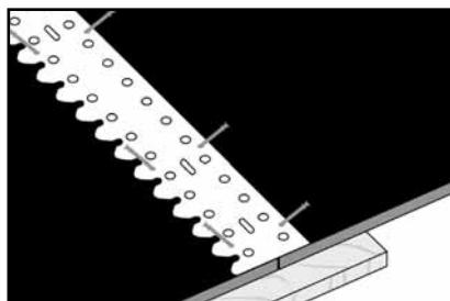
**2.** Support belt ends with wood plank. Nail Flexco Templet in position with belt ends tight against lugs.
