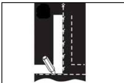
**1.** Square belt ends using centerline method. Cut belt ends using Flexco 840 Series Belt Cutter.
