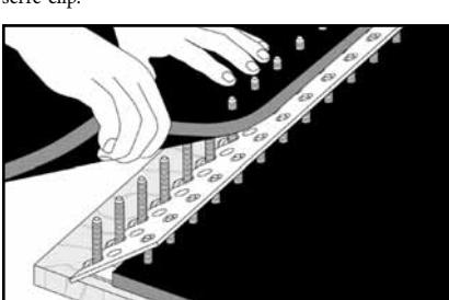
**6.** Align bolts with templet teeth and place the other belt end over bolts. Remove templet.
