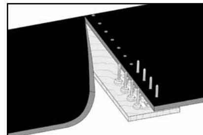
**5.** Fold one belt end back and insert bolts in one row of holes.
