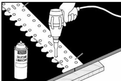
**NOTE:** A  $\frac{1}{2}$ " square drive electric impact wrench with Flexco 5552 Quick Change Chuck will speed hole boring operation.
