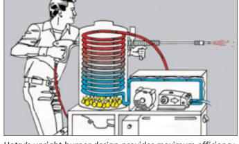
Hotsy's upright burner design provides maximum efficiency for fast heating, easy venting in indoor applications, plus excellent fuel economy.
