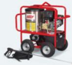
**Model 781SS** 2.5 GPM @ 2000 PSI; 6 HP Robin Subaru OHV gas engine; 12V DC oil fired water heater (Battery not required)
